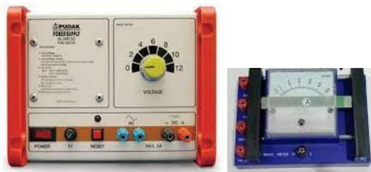
**Gambar 3.7.** Power supply variabel diskret, dan basic meter
